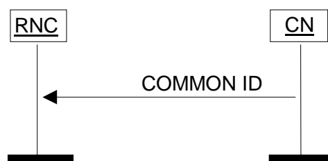
Figure 17: Common ID procedure. Successful operation.
