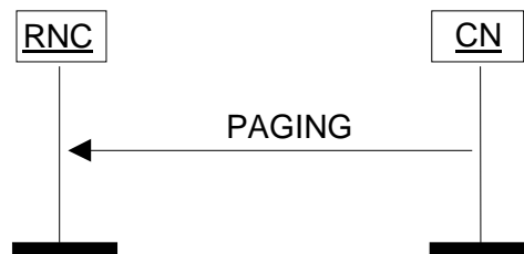
Figure 16: Paging procedure. Successful operation.
