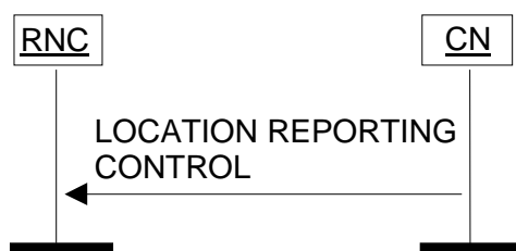
Figure 21: Location Reporting Control procedure. Successful operation.
