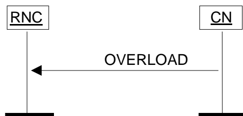
Figure 27: Overload at the CN. Successful operation.
