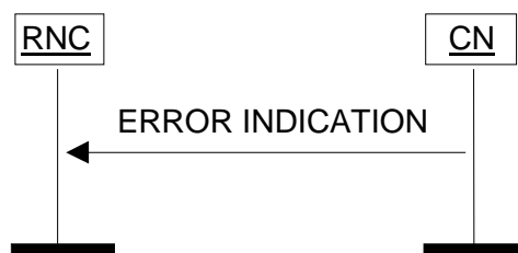
Figure 31: Error Indication procedure, CN originated. Successful operation.
