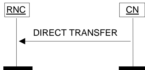
Figure 25: Direct Transfer, CN originated. Successful operation.
