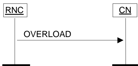
Figure 28: Overload at the UTRAN. Successful operation.
