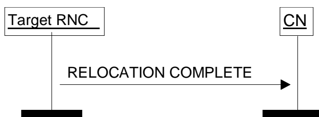
Figure 10: Relocation Complete procedure. Successful operation.
