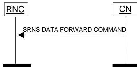
Figure 13: SRNS Data Forwarding Initiation procedure. Successful operation.
