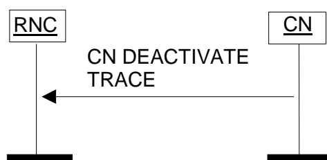
Figure 33: CN Deactivate Trace procedure. Successful operation.
