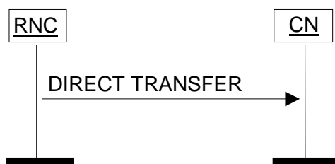
Figure 26: Direct Transfer, RNC originated. Successful operation.
