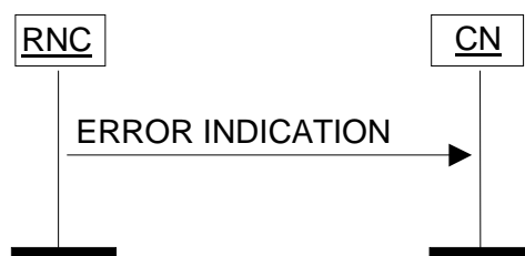
Figure 32: Error Indication procedure, RNC originated. Successful operation.
