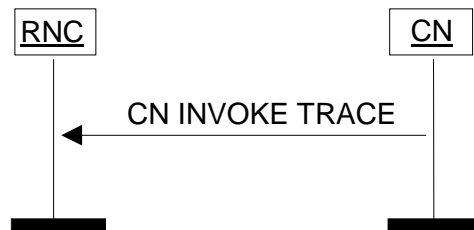
Figure 18: CN Invoke Trace procedure. Successful operation.
