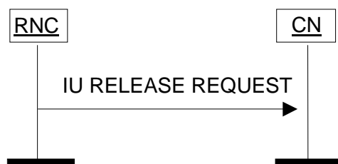
Figure 3: Iu Release Request procedure. Successful operation.
