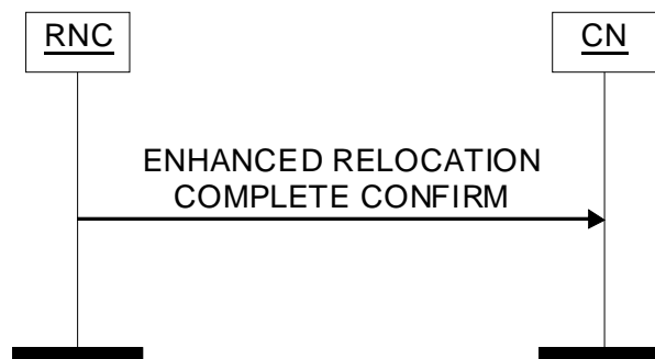
Figure 60: Enhanced Relocation Complete Confirm procedure. Successful operation.
