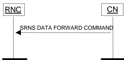
Figure 13: SRNS Data Forwarding Initiation procedure. Successful operation.
