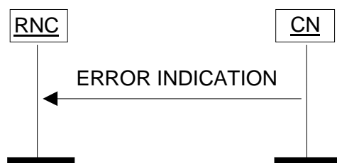
Figure 31: Error Indication procedure, CN originated. Successful operation.
