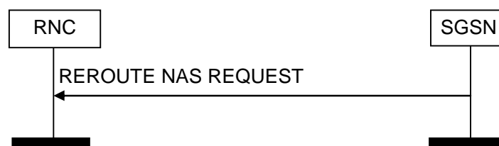
Figure 64: Reroute NAS Request procedure: Successful operation.
