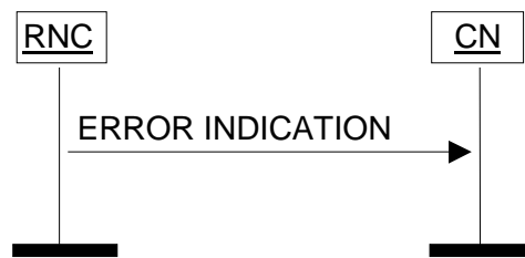
Figure 32: Error Indication procedure, RNC originated. Successful operation.
