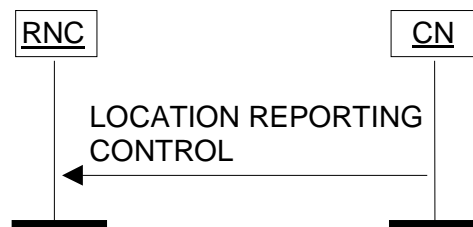
Figure 21: Location Reporting Control procedure. Successful operation.
