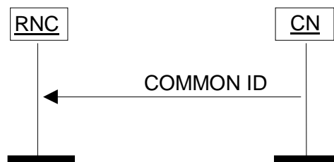
Figure 17: Common ID procedure. Successful operation.
