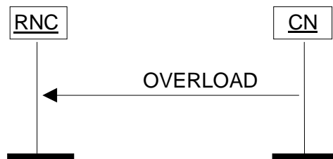
Figure 27: Overload at the CN. Successful operation.
