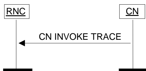
Figure 18: CN Invoke Trace procedure. Successful operation.
