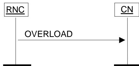
Figure 28: Overload at the UTRAN. Successful operation.
