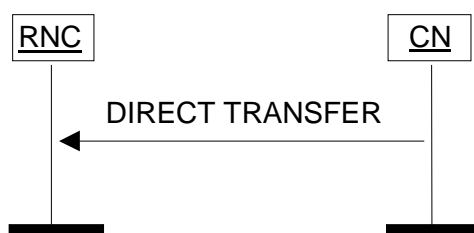
Figure 25: Direct Transfer, CN originated. Successful operation.
