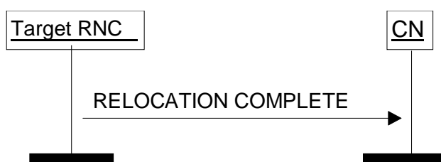
Figure 10: Relocation Complete procedure. Successful operation.
