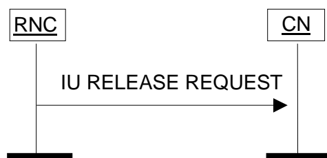
Figure 3: Iu Release Request procedure. Successful operation.
