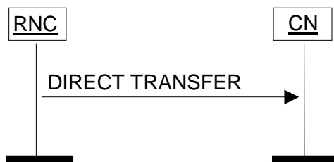
Figure 26: Direct Transfer, RNC originated. Successful operation.
