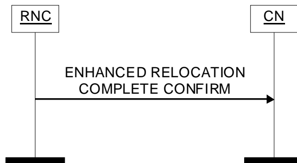
Figure 60: Enhanced Relocation Complete Confirm procedure. Successful operation.
