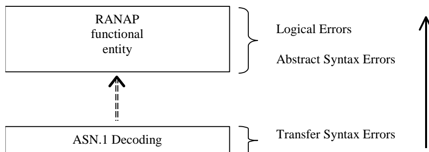
Figure 36: Protocol Errors in RANAP.
