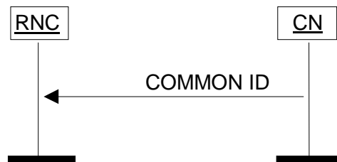
Figure 17: Common ID procedure. Successful operation.
