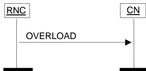
Figure 28: Overload at the UTRAN. Successful operation.
