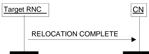
Figure 10: Relocation Complete procedure. Successful operation.
