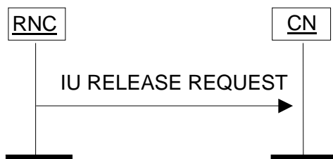
Figure 3: Iu Release Request procedure. Successful operation.
