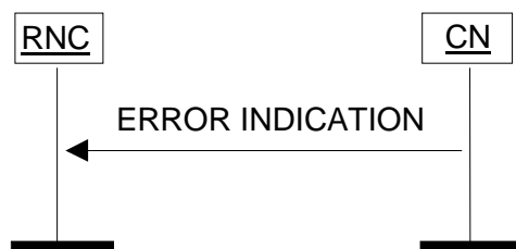
Figure 31: Error Indication procedure, CN originated. Successful operation.
