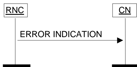
Figure 32: Error Indication procedure, RNC originated. Successful operation.
