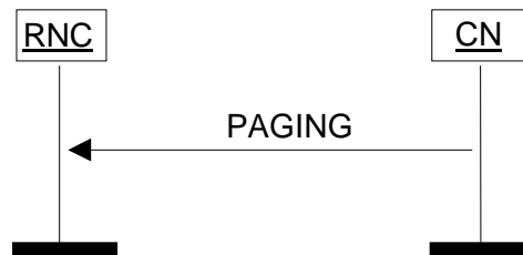
Figure 16: Paging procedure. Successful operation.
