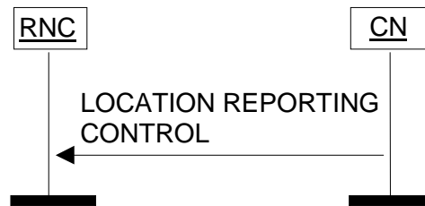
Figure 21: Location Reporting Control procedure. Successful operation.
