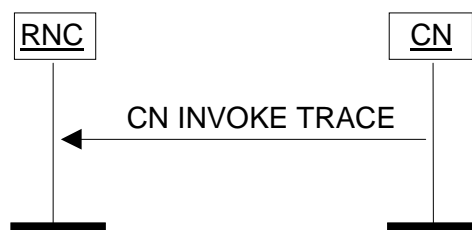
Figure 18: CN Invoke Trace procedure. Successful operation.
