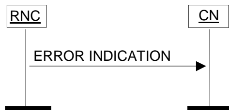
Figure 32: Error Indication procedure, RNC originated. Successful operation.
