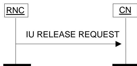
Figure 3: Iu Release Request procedure. Successful operation.
