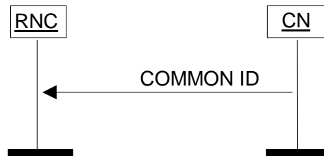
Figure 17: Common ID procedure. Successful operation.
