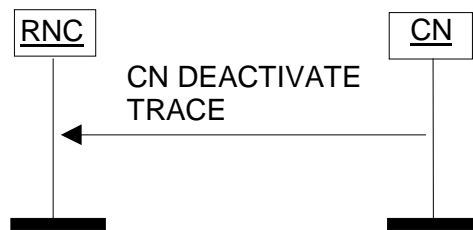
Figure 33: CN Deactivate Trace procedure. Successful operation.
