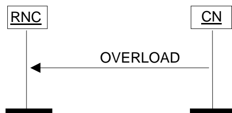
Figure 27: Overload at the CN. Successful operation.
