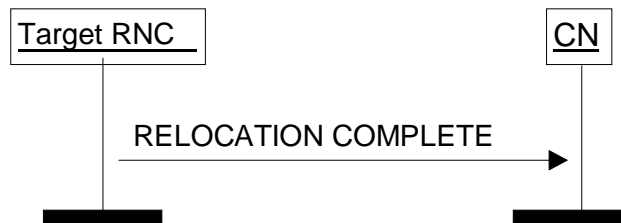
Figure 10: Relocation Complete procedure. Successful operation.
