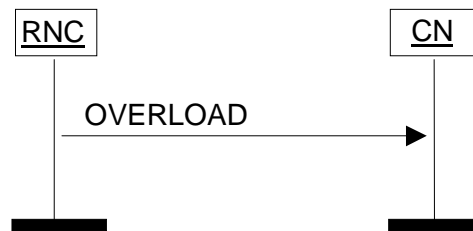
Figure 28: Overload at the UTRAN. Successful operation.
