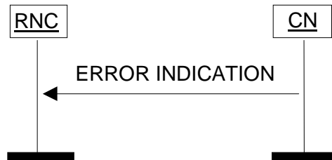
Figure 31: Error Indication procedure, CN originated. Successful operation.
