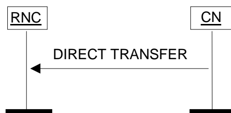
Figure 25: Direct Transfer, CN originated. Successful operation.
