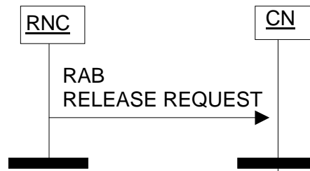
Figure 2: RAB Release Request procedure. Successful operation.
