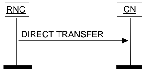
Figure 26: Direct Transfer, RNC originated. Successful operation.
