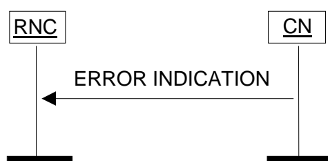
Figure 31: Error Indication procedure, CN originated. Successful operation.
