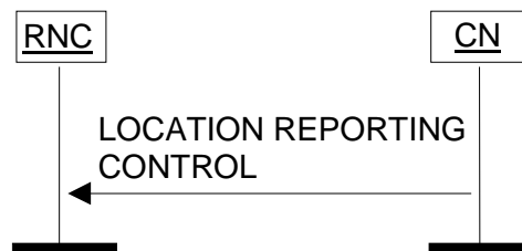
Figure 21: Location Reporting Control procedure. Successful operation.
