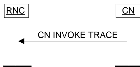
Figure 18: CN Invoke Trace procedure. Successful operation.
