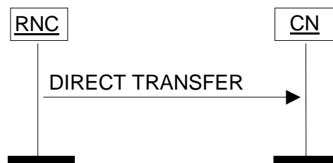
Figure 26: Direct Transfer, RNC originated. Successful operation.
