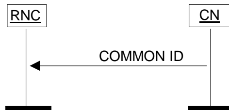
Figure 17: Common ID procedure. Successful operation.
