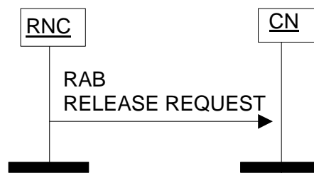
Figure 2: RAB Release Request procedure. Successful operation.
