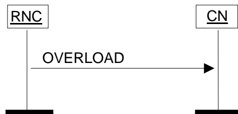
Figure 28: Overload at the UTRAN. Successful operation.
