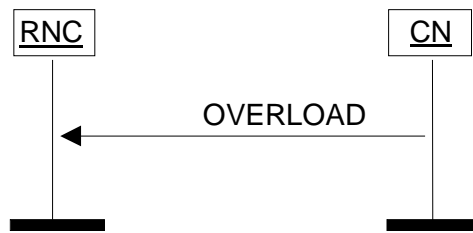
Figure 27: Overload at the CN. Successful operation.
