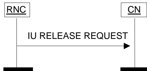
Figure 3: Iu Release Request procedure. Successful operation.
