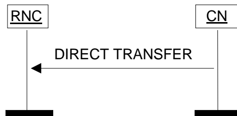
Figure 25: Direct Transfer, CN originated. Successful operation.
