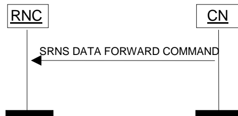
Figure 13: SRNS Data Forwarding Initiation procedure. Successful operation.
