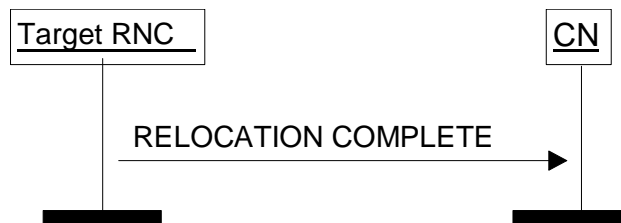
Figure 10: Relocation Complete procedure. Successful operation.
