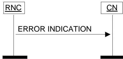
Figure 32: Error Indication procedure, RNC originated. Successful operation.
