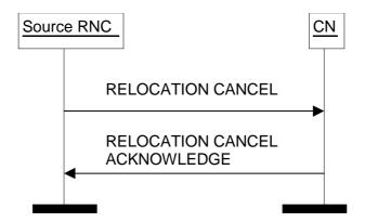
Figure 11: Relocation Cancel procedure. Successful operation.
