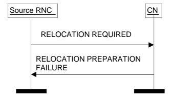
Figure 6: Relocation Preparation procedure. Unsuccessful operation.
