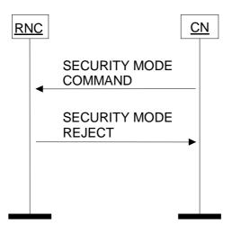
Figure 20: Security Mode Control procedure. Unsuccessful operation.
