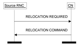
Figure 5: Relocation Preparation procedure. Successful operation.
