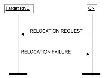
Figure 8: Relocation Resource Allocation procedure: Unsuccessful operation.
