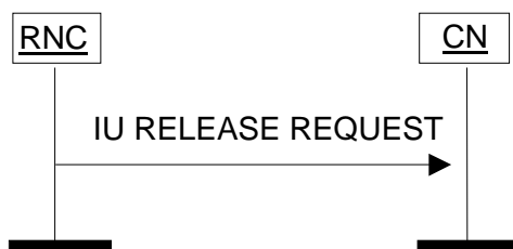
Figure 3: Iu Release Request procedure. Successful operation.
