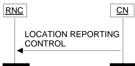
Figure 21: Location Reporting Control procedure. Successful operation.
