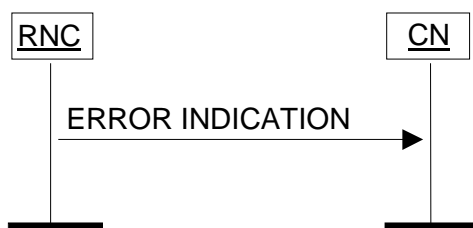
Figure 32: Error Indication procedure, RNC originated. Successful operation.
