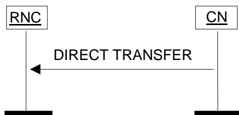
Figure 25: Direct Transfer, CN originated. Successful operation.
