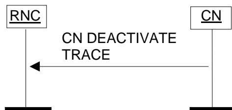
Figure 33: CN Deactivate Trace procedure. Successful operation.
