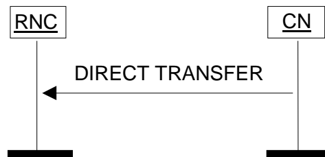
Figure 25: Direct Transfer, CN originated. Successful operation.
