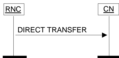
Figure 26: Direct Transfer, RNC originated. Successful operation.
