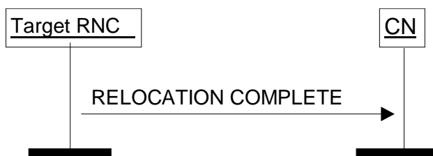
Figure 10: Relocation Complete procedure. Successful operation.
