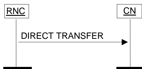
Figure 26: Direct Transfer, RNC originated. Successful operation.
