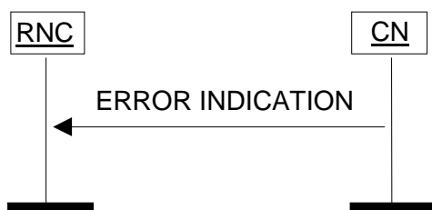
Figure 31: Error Indication procedure, CN originated. Successful operation.
