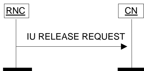
Figure 3: Iu Release Request procedure. Successful operation.
