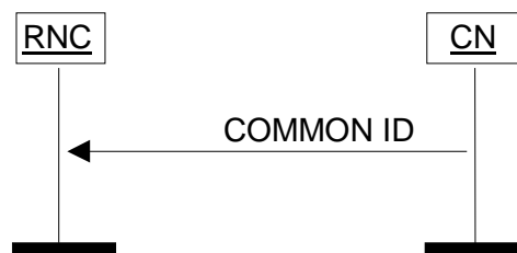
Figure 17: Common ID procedure. Successful operation.
