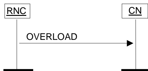
Figure 28: Overload at the UTRAN. Successful operation.
