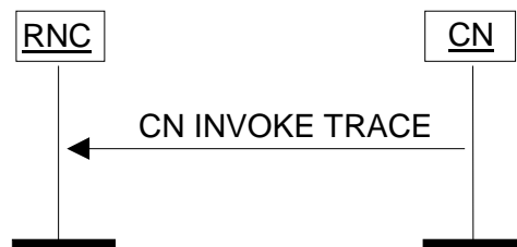
Figure 18: CN Invoke Trace procedure. Successful operation.
