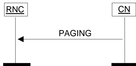
Figure 16: Paging procedure. Successful operation.
