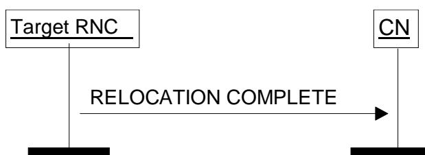
Figure 10: Relocation Complete procedure. Successful operation.
