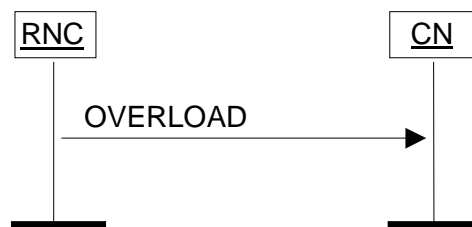
Figure 28: Overload at the UTRAN. Successful operation.
