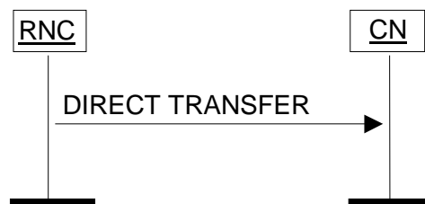
Figure 26: Direct Transfer, RNC originated. Successful operation.
