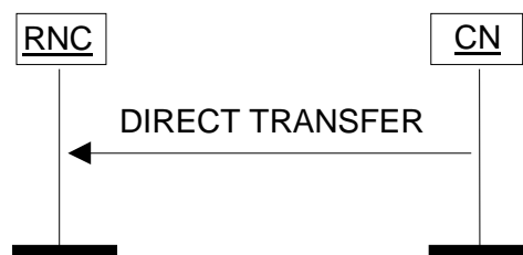
Figure 25: Direct Transfer, CN originated. Successful operation.
