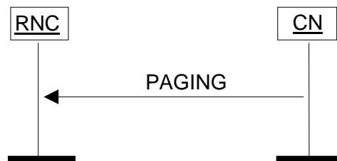
Figure 16: Paging procedure. Successful operation.
