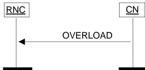
Figure 27: Overload at the CN. Successful operation.
