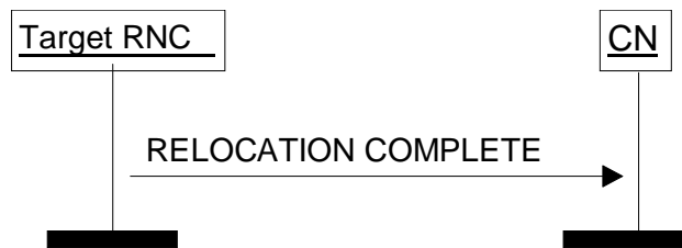
Figure 10: Relocation Complete procedure. Successful operation.
