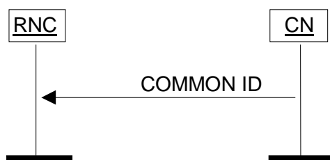
Figure 17: Common ID procedure. Successful operation.
