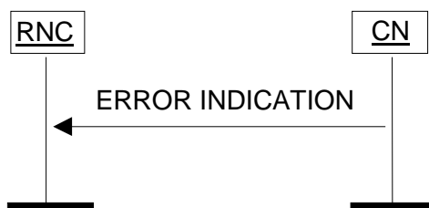
Figure 31: Error Indication procedure, CN originated. Successful operation.
