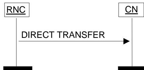
Figure 26: Direct Transfer, RNC originated. Successful operation.
