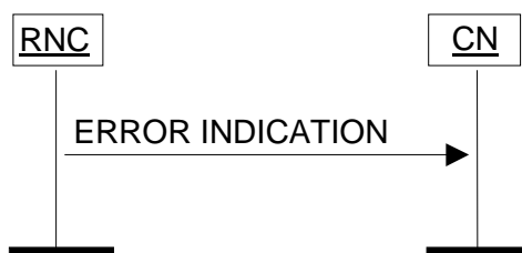
Figure 32: Error Indication procedure, RNC originated. Successful operation.
