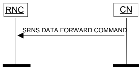
Figure 13: SRNS Data Forwarding Initiation procedure. Successful operation.
