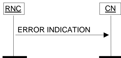
Figure 32: Error Indication procedure, RNC originated. Successful operation.
