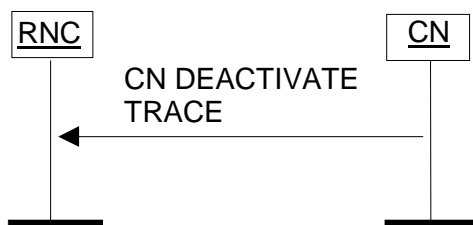
Figure 33: CN Deactivate Trace procedure. Successful operation.
