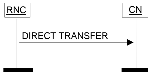
Figure 26: Direct Transfer, RNC originated. Successful operation.
