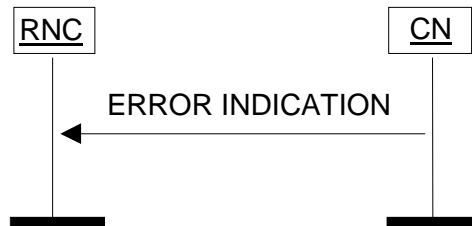
Figure 31: Error Indication procedure, CN originated. Successful operation.
