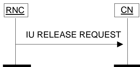
Figure 3: Iu Release Request procedure. Successful operation.
