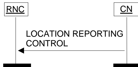
Figure 21: Location Reporting Control procedure. Successful operation.
