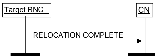
Figure 10: Relocation Complete procedure. Successful operation.
