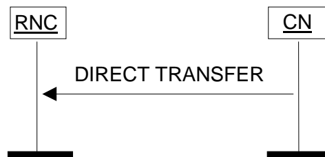
Figure 25: Direct Transfer, CN originated. Successful operation.
