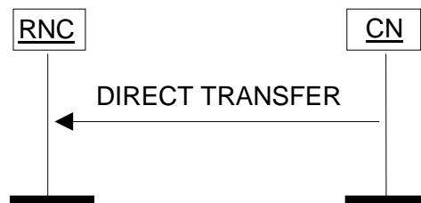
Figure 25: Direct Transfer, CN originated. Successful operation.
