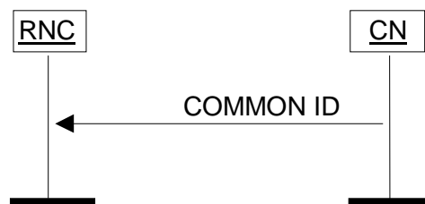
Figure 17: Common ID procedure. Successful operation.
