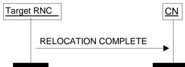
Figure 10: Relocation Complete procedure. Successful operation.
