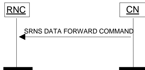
Figure 13: SRNS Data Forwarding Initiation procedure. Successful operation.
