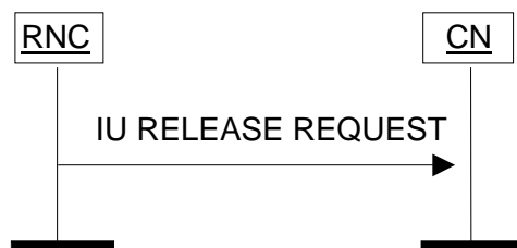
Figure 3: Iu Release Request procedure. Successful operation.
