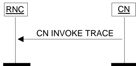
Figure 18: CN Invoke Trace procedure. Successful operation.
