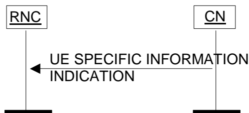
Figure 41: UE Specific Information procedure. Successful operation.
