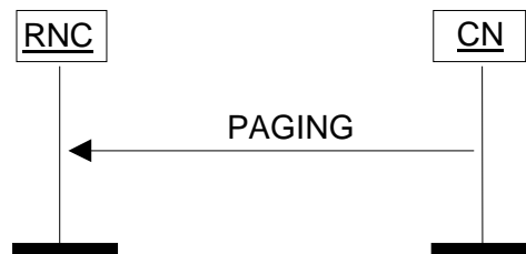
Figure 16: Paging procedure. Successful operation.
