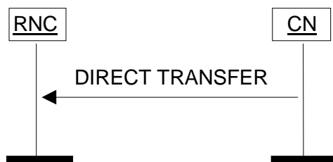
Figure 25: Direct Transfer, CN originated. Successful operation.
