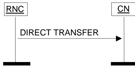
Figure 26: Direct Transfer, RNC originated. Successful operation.
