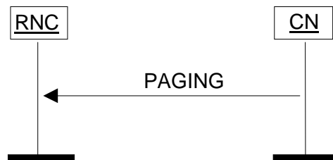
Figure 16: Paging procedure. Successful operation.
