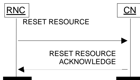
Figure 34: RNC initiated Reset Resource procedure. Successful operation.
