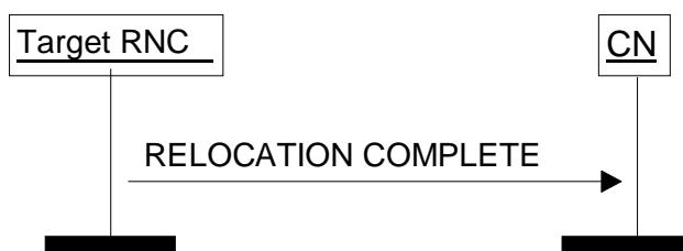
Figure 10: Relocation Complete procedure. Successful operation.
