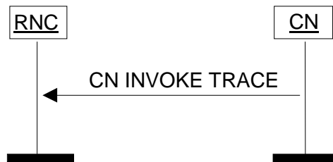
Figure 18: CN Invoke Trace procedure. Successful operation.
