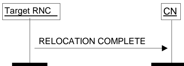
Figure 10: Relocation Complete procedure. Successful operation.
