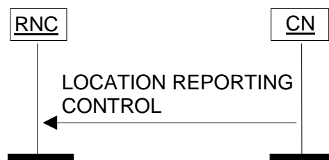
Figure 21: Location Reporting Control procedure. Successful operation.
