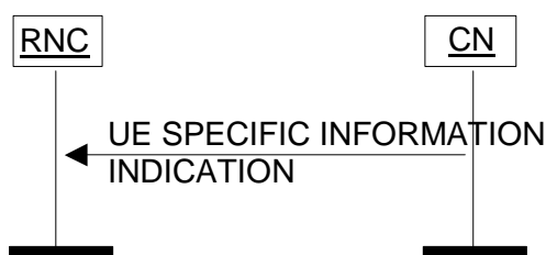
Figure 41: UE Specific Information procedure. Successful operation.
