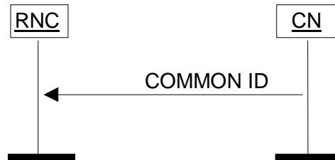
Figure 17: Common ID procedure. Successful operation.
