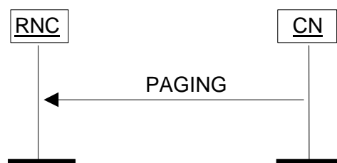
Figure 16: Paging procedure. Successful operation.
