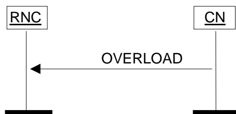
Figure 27: Overload at the CN. Successful operation.
