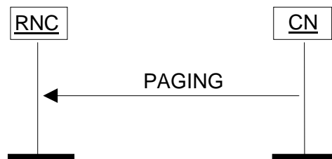
Figure 16: Paging procedure. Successful operation.
