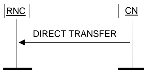
Figure 25: Direct Transfer, CN originated. Successful operation.
