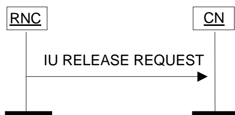
Figure 3: Iu Release Request procedure. Successful operation.
