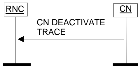
Figure 33: CN Deactivate Trace procedure. Successful operation.
