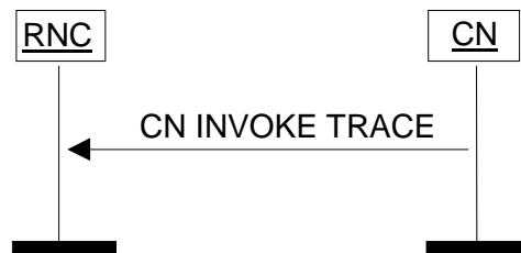
Figure 18: CN Invoke Trace procedure. Successful operation.
