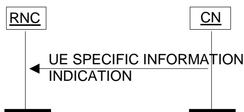
Figure 41: UE Specific Information procedure. Successful operation.
