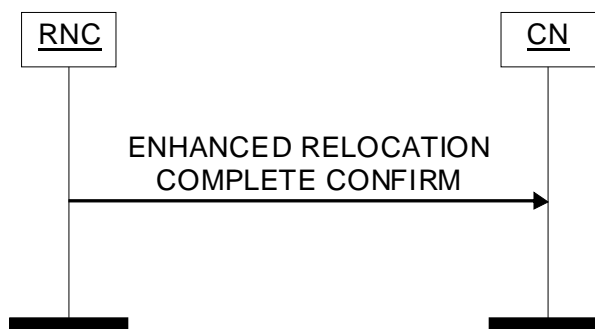
Figure 70: Enhanced Relocation Complete Confirm procedure. Successful operation.
