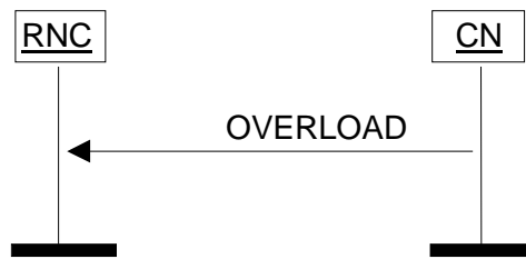
Figure 27: Overload at the CN. Successful operation.
