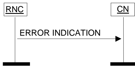
Figure 32: Error Indication procedure, RNC originated. Successful operation.
