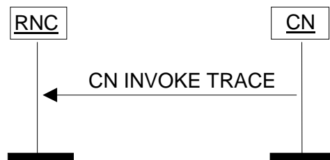
Figure 18: CN Invoke Trace procedure. Successful operation.
