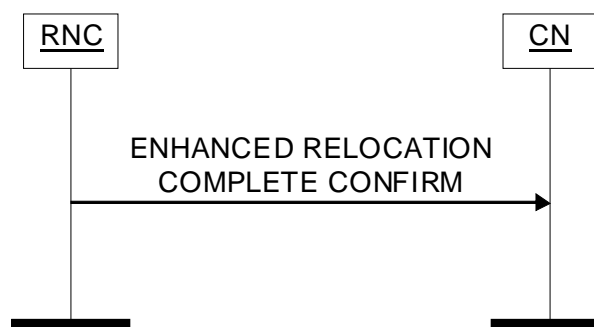
Figure 70: Enhanced Relocation Complete Confirm procedure. Successful operation.
