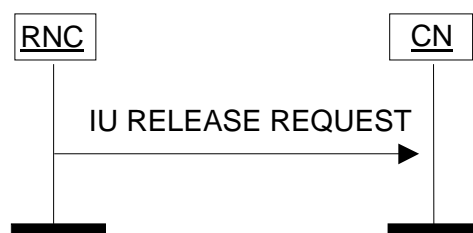
Figure 3: Iu Release Request procedure. Successful operation.
