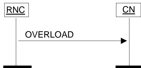
Figure 28: Overload at the UTRAN. Successful operation.
