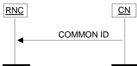
Figure 17: Common ID procedure. Successful operation.
