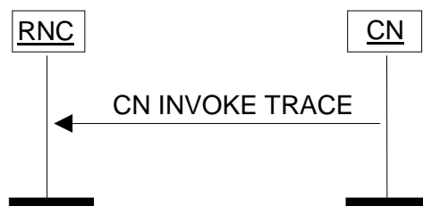
Figure 18: CN Invoke Trace procedure. Successful operation.
