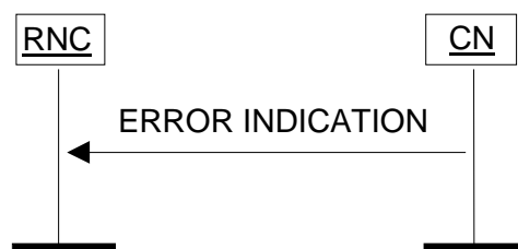
Figure 31: Error Indication procedure, CN originated. Successful operation.
