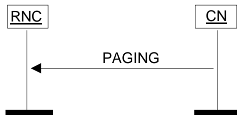
Figure 16: Paging procedure. Successful operation.
