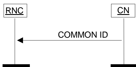
Figure 17: Common ID procedure. Successful operation.
