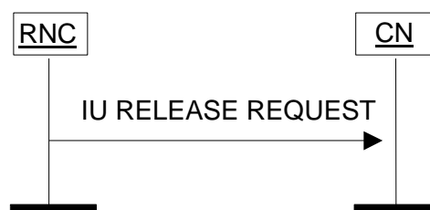
Figure 3: Iu Release Request procedure. Successful operation.
