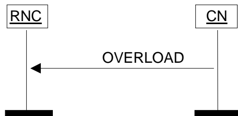
Figure 27: Overload at the CN. Successful operation.
