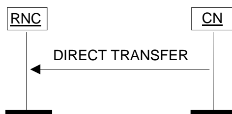
Figure 25: Direct Transfer, CN originated. Successful operation.
