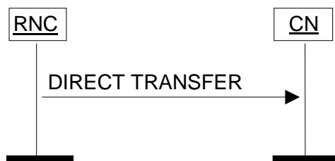
Figure 26: Direct Transfer, RNC originated. Successful operation.
