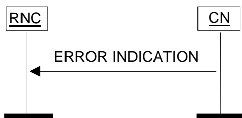
Figure 31: Error Indication procedure, CN originated. Successful operation.
