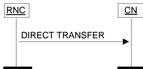
Figure 26: Direct Transfer, RNC originated. Successful operation.
