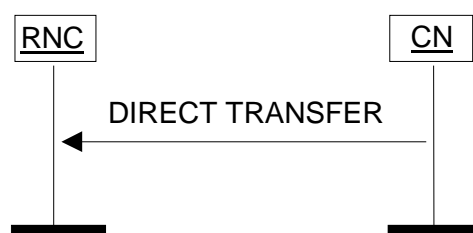
Figure 25: Direct Transfer, CN originated. Successful operation.
