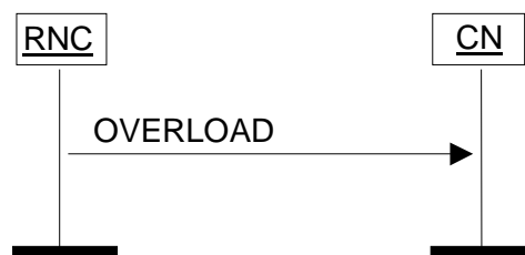
Figure 28: Overload at the UTRAN. Successful operation.
