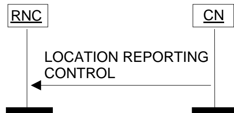
Figure 21: Location Reporting Control procedure. Successful operation.
