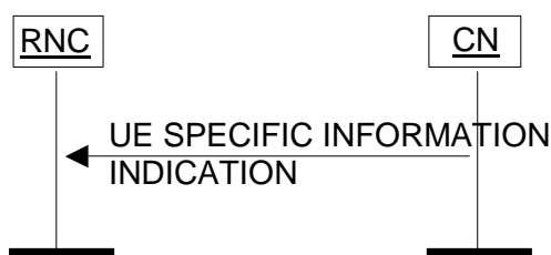
Figure 41: UE Specific Information procedure. Successful operation.
