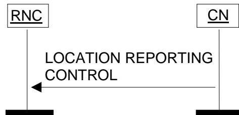
Figure 21: Location Reporting Control procedure. Successful operation.
