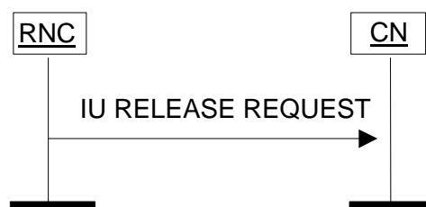
Figure 3: Iu Release Request procedure. Successful operation.
