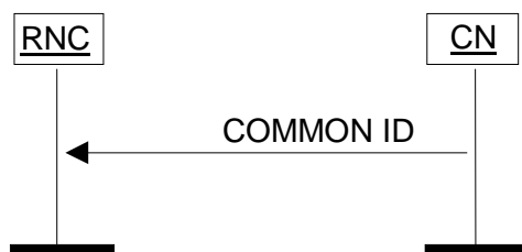
Figure 17: Common ID procedure. Successful operation.
