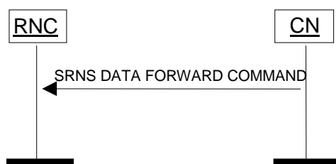
Figure 13: SRNS Data Forwarding Initiation procedure. Successful operation.
