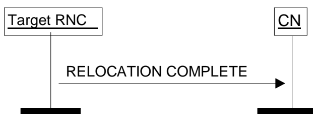
Figure 10: Relocation Complete procedure. Successful operation.
