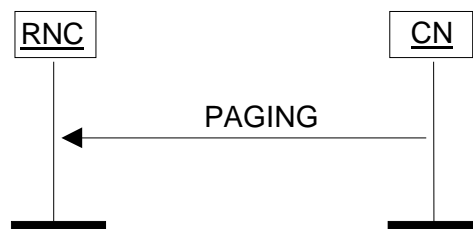
Figure 16: Paging procedure. Successful operation.
