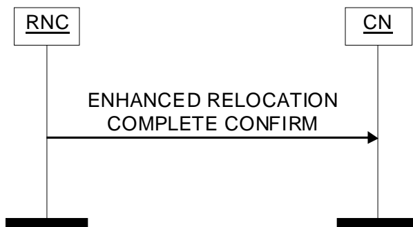
Figure 70: Enhanced Relocation Complete Confirm procedure. Successful operation.
