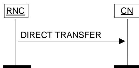
Figure 26: Direct Transfer, RNC originated. Successful operation.
