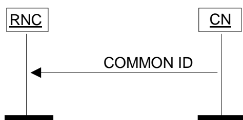
Figure 17: Common ID procedure. Successful operation.
