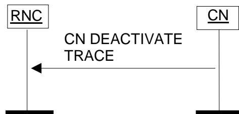
Figure 33: CN Deactivate Trace procedure. Successful operation.
