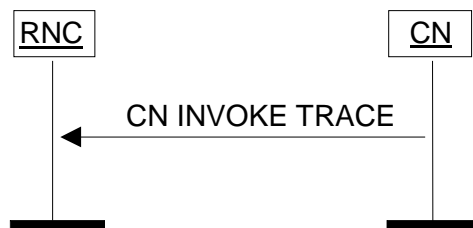
Figure 18: CN Invoke Trace procedure. Successful operation.
