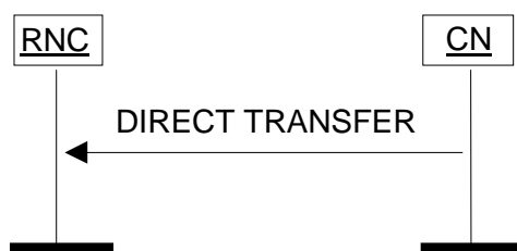
Figure 25: Direct Transfer, CN originated. Successful operation.
