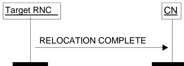
Figure 10: Relocation Complete procedure. Successful operation.
