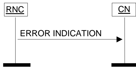
Figure 32: Error Indication procedure, RNC originated. Successful operation.
