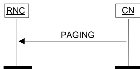
Figure 16: Paging procedure. Successful operation.
