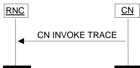
Figure 18: CN Invoke Trace procedure. Successful operation.
