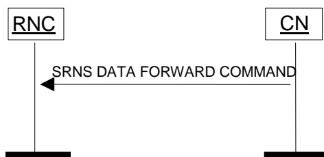
Figure 13: SRNS Data Forwarding Initiation procedure. Successful operation.
