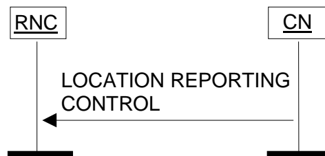
Figure 21: Location Reporting Control procedure. Successful operation.
