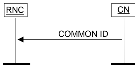
Figure 17: Common ID procedure. Successful operation.
