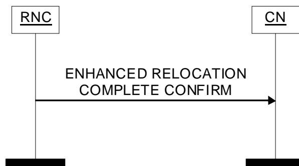
Figure 70: Enhanced Relocation Complete Confirm procedure. Successful operation.
