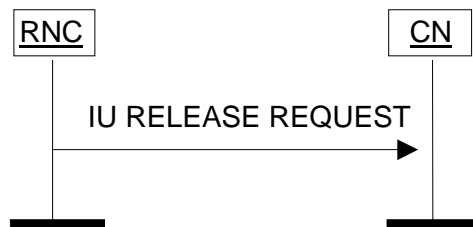
Figure 3: Iu Release Request procedure. Successful operation.
