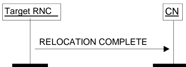
Figure 10: Relocation Complete procedure. Successful operation.
