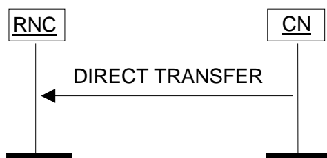
Figure 25: Direct Transfer, CN originated. Successful operation.
