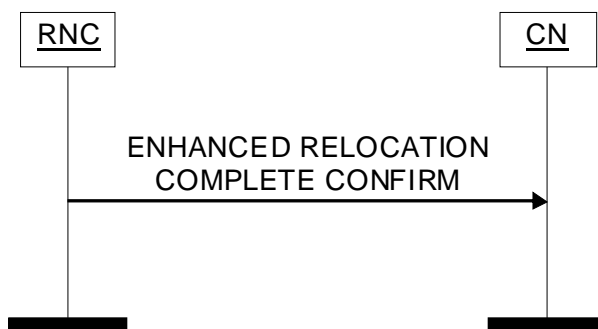
Figure 70: Enhanced Relocation Complete Confirm procedure. Successful operation.
