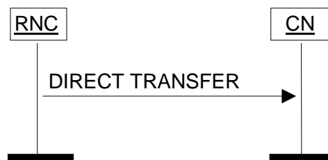
Figure 26: Direct Transfer, RNC originated. Successful operation.
