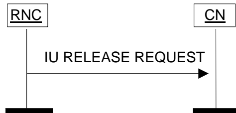
Figure 3: Iu Release Request procedure. Successful operation.
