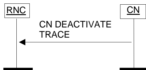
Figure 33: CN Deactivate Trace procedure. Successful operation.
