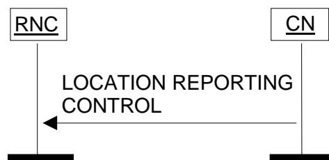
Figure 21: Location Reporting Control procedure. Successful operation.
