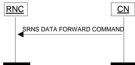
Figure 13: SRNS Data Forwarding Initiation procedure. Successful operation.
