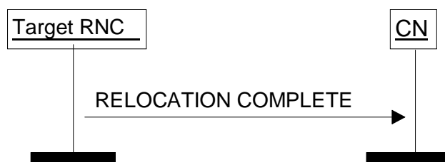
Figure 10: Relocation Complete procedure. Successful operation.
