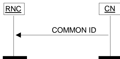
Figure 17: Common ID procedure. Successful operation.
