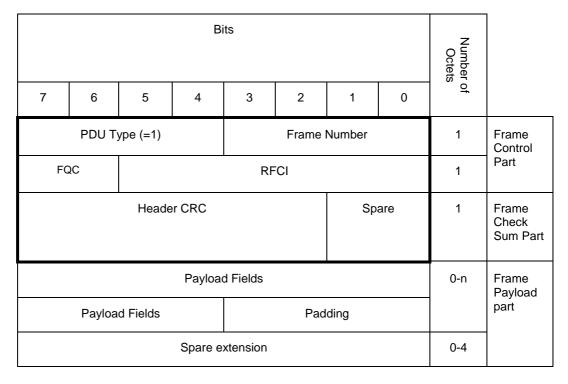
Figure 20: lu UP PDU Type 1 Format
