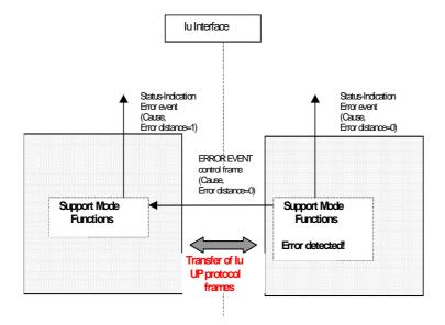
Figure 29: Internal error
