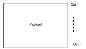
Figure 4: Frame format for transparent mode
