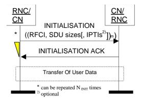
Figure 9: Successful Initialisation of Iu UP for m RFCIs
