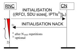
Figure 10: Unsuccessful initialisation of lu UP: 1) N <sub>INIT</sub> negative acknowledgement or 2) N <sub>INIT</sub> expiries of timer T<sub>INIT</sub>
