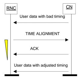
Figure 15a: Successful Time Alignment
