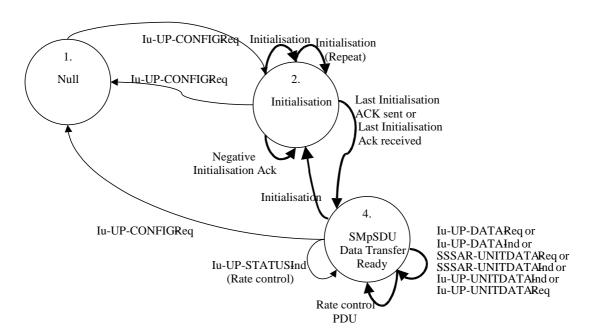
Figure B.2: Protocol state model for support mode
