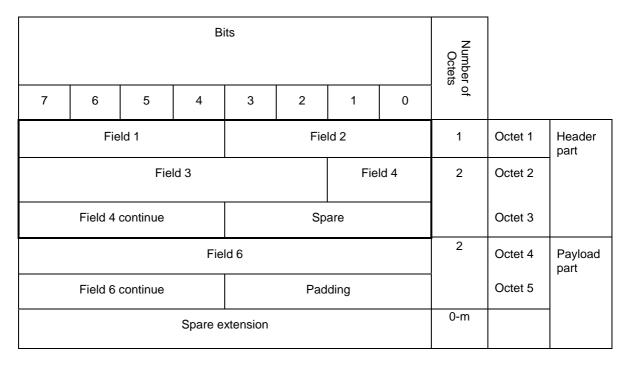
Figure 18: Example frame format
