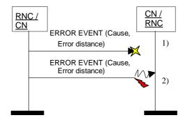
Figure 16c: Unsuccessful Transfer of ERROR EVENT control frame: 1) Frame loss 2) Corrupted Frame
