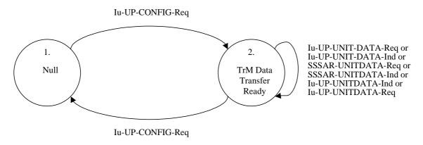
Figure B.1: Protocol state model for transparent mode
