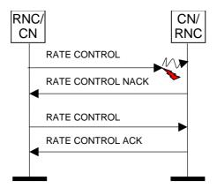
Figure 13a: Negative Acknowledgement received from the peer
