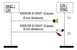
Figure 16c: Unsuccessful Transfer of ERROR EVENT control frame: 1) Frame loss 2) Corrupted
