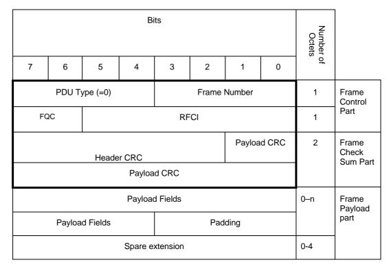
Figure 19: Iu UP PDU Type 0 Format
