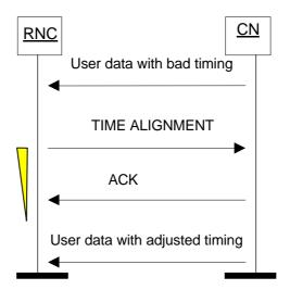
Figure 15a: Successful Time Alignment
