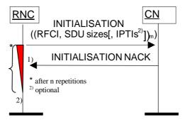
Figure 10: Unsuccessful initialisation of lu UP: 1) N <sub>INIT</sub> negative acknowledgement or 2) N <sub>INIT</sub> expiries of timer T<sub>INIT</sub>
