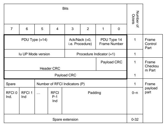
Figure 25: Iu UP PDU Type 14 Format used for Rate Control
