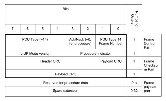
Figure 21: Iu UP PDU Type 14 Format for procedure sending
