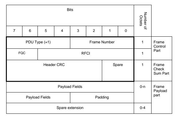
Figure 20: Iu UP PDU Type 1 Format
