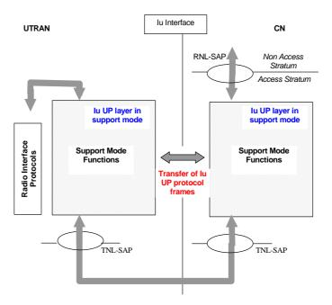
Figure 3: lu UP protocol layer in support mode occurrence over lu interface
