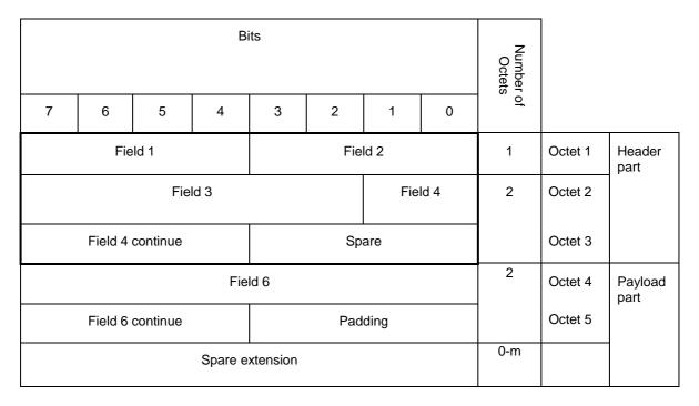
Figure 18: Example frame format
