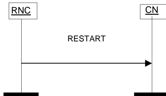
Figure 11: Restart Indication Procedure: Successful Operation
