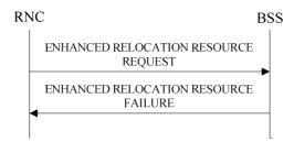
Figure 4C: Enhanced Relocation Resource Allocation Procedure, Unsuccessful Operation
