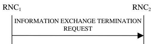
Figure 30I: Information Exchange Termination procedure, Successful Operation
