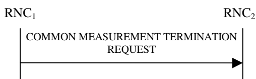
Figure 30D: Common Measurement Termination procedure, Successful Operation
