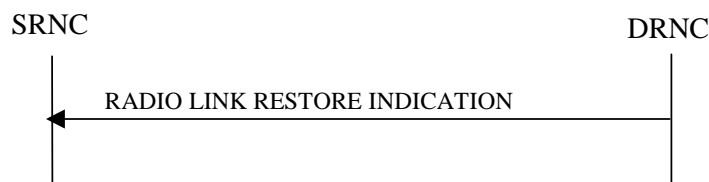
Figure 19: Radio Link Restoration procedure, Successful Operation
