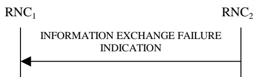
Figure 30J: Information Exchange Failure procedure, Successful Operation
