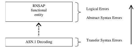
Figure 34: Protocol Errors in RNSAP
