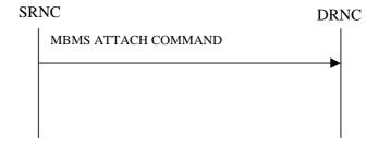
Figure 31: MBMS Attach procedure, Successful Operation
