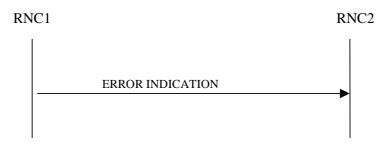
Figure 30: Error Indication procedure, Successful Operation
