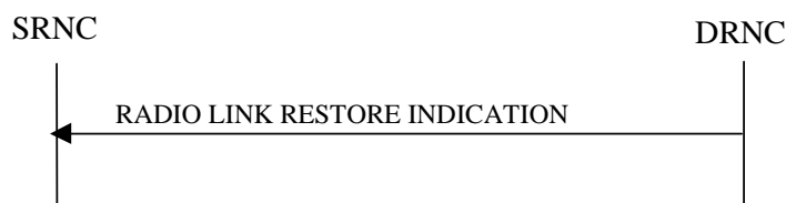
Figure 19: Radio Link Restoration procedure, Successful Operation
