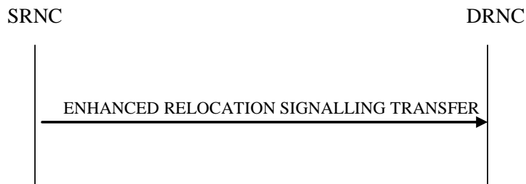
Figure 26P: Enhanced Relocation Signalling Transfer procedure, Successful Operation
