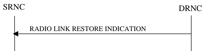
Figure 19: Radio Link Restoration procedure, Successful Operation
