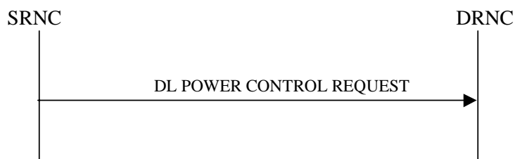
Figure 25: Downlink Power Control procedure, Successful Operation
