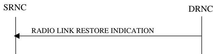
Figure 19: Radio Link Restoration procedure, Successful Operation
