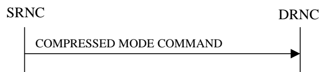
Figure 26: Compressed Mode Command procedure, Successful Operation
