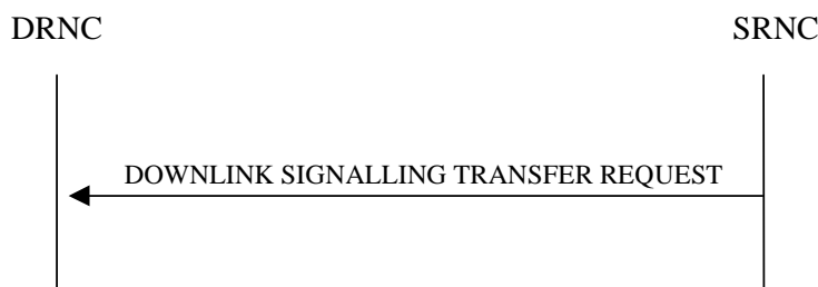
Figure 2: Downlink Signalling Transfer procedure, Successful Operation
