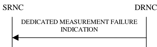
Figure 24: Dedicated Measurement Failure procedure, Successful Operation
