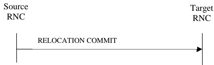
Figure 3: Relocation Commit procedure, Successful Operation
