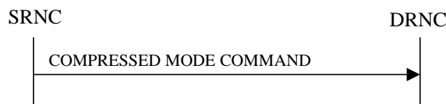
Figure 26: Compressed Mode Command procedure, Successful Operation
