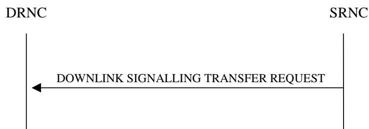
Figure 2: Downlink Signalling Transfer procedure, Successful Operation
