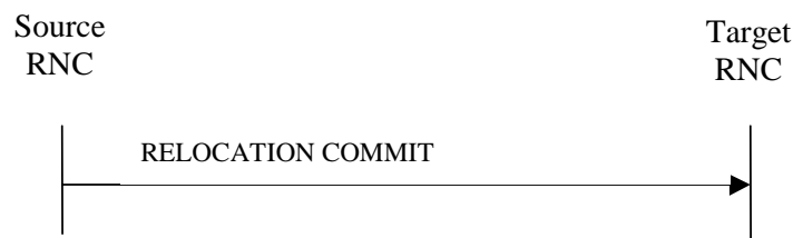
Figure 3: Relocation Commit procedure, Successful Operation
