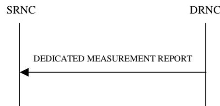
Figure 22: Measurement Reporting procedure, Successful Operation
