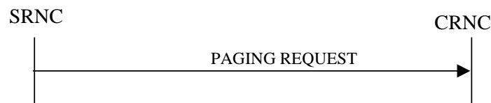
Figure 4: Paging procedure, Successful Operation
