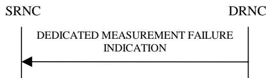
Figure 24: Measurement Failure procedure, Successful Operation
