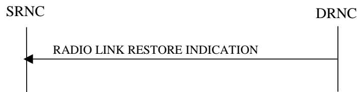
Figure 19: RL Restoration procedure, Successful Operation
