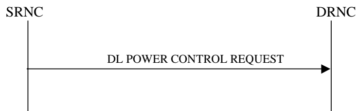
Figure 25: Downlink Power Control procedure, Successful Operation
