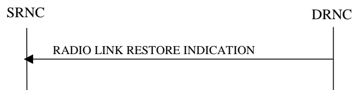
Figure 19: RL Restoration procedure, Successful Operation
