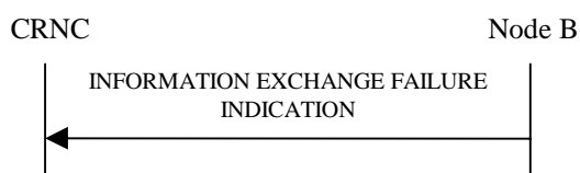
Figure 30J: Information Exchange Failure procedure, Successful Operation
