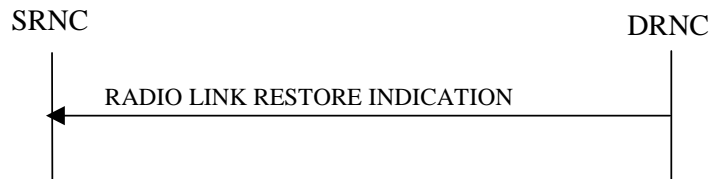
Figure 19: RL Restoration procedure, Successful Operation
