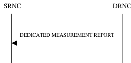
Figure 22: Dedicated Measurement Reporting procedure, Successful Operation
