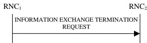
Figure 30I: Information Exchange Termination procedure, Successful Operation
