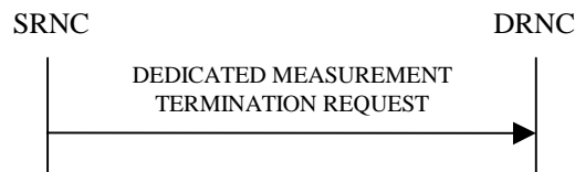
Figure 23: Dedicated Measurement Termination procedure, Successful Operation
