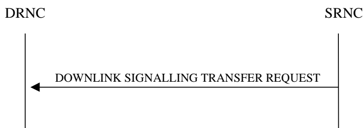
Figure 2: Downlink Signalling Transfer procedure, Successful Operation
