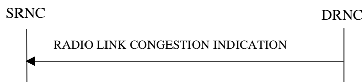
Figure 26C: Radio Link Congestion procedure, Successful Operation
