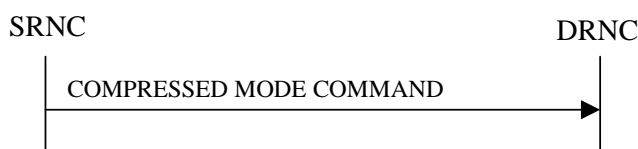
Figure 26: Compressed Mode Command procedure, Successful Operation
