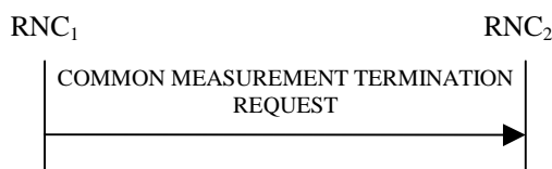
Figure 30D: Common Measurement Termination procedure, Successful Operation
