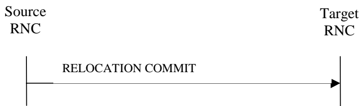
Figure 3: Relocation Commit procedure, Successful Operation
