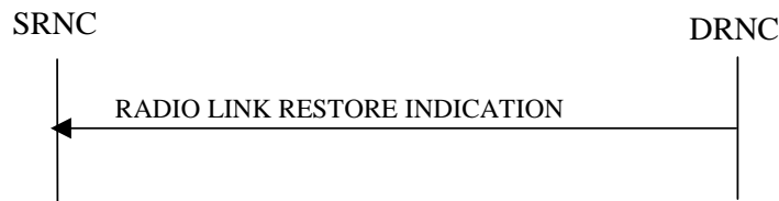
Figure 19: Radio Link Restoration procedure, Successful Operation
