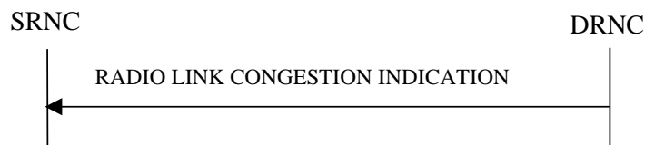
Figure 26C: Radio Link Congestion procedure, Successful Operation
