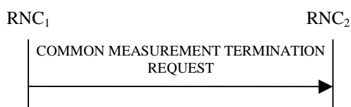
Figure 30D: Common Measurement Termination procedure, Successful Operation
