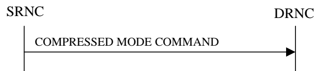
Figure 26: Compressed Mode Command procedure, Successful Operation
