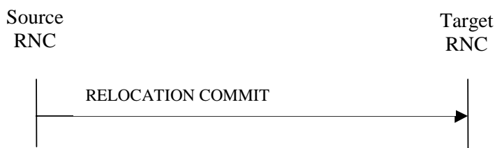
Figure 3: Relocation Commit procedure, Successful Operation
