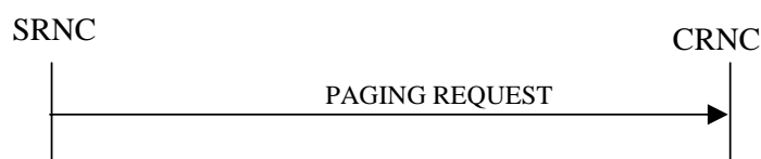
Figure 4: Paging procedure, Successful Operation
