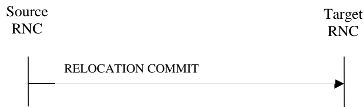
Figure 3: Relocation Commit procedure, Successful Operation
