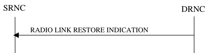
Figure 19: Radio Link Restoration procedure, Successful Operation
