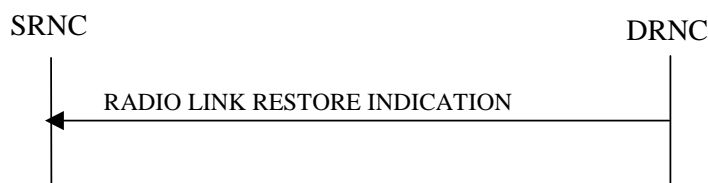
Figure 19: Radio Link Restoration procedure, Successful Operation
