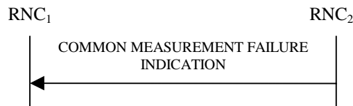
Figure 30E: Common Measurement Failure procedure, Successful Operation
