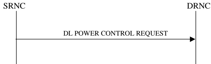
Figure 25: Downlink Power Control procedure, Successful Operation
