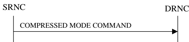
Figure 26: Compressed Mode Command procedure, Successful Operation
