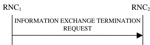
Figure 30I: Information Exchange Termination procedure, Successful Operation
