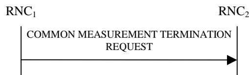
Figure 30D: Common Measurement Termination procedure, Successful Operation
