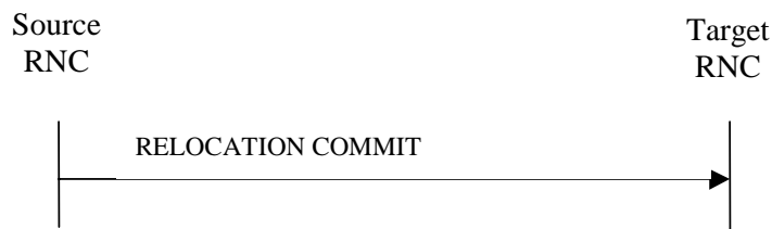
Figure 3: Relocation Commit procedure, Successful Operation
