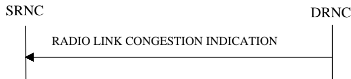
Figure 26C: Radio Link Congestion procedure, Successful Operation
