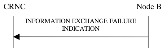
Figure 30J: Information Exchange Failure procedure, Successful Operation
