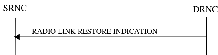
Figure 19: Radio Link Restoration procedure, Successful Operation
