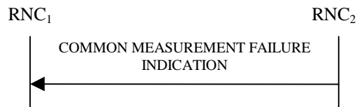
Figure 30E: Common Measurement Failure procedure, Successful Operation
