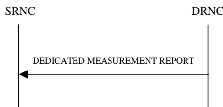
Figure 22: Dedicated Measurement Reporting procedure, Successful Operation
