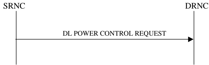
Figure 25: Downlink Power Control procedure, Successful Operation
