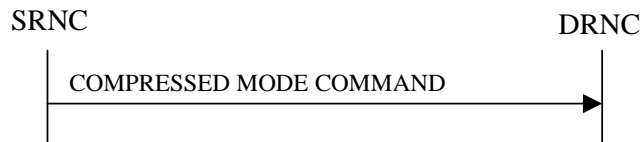
Figure 26: Compressed Mode Command procedure, Successful Operation
