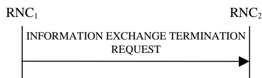
Figure 30I: Information Exchange Termination procedure, Successful Operation
