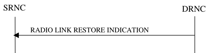
Figure 19: Radio Link Restoration procedure, Successful Operation
