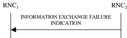
Figure 30J: Information Exchange Failure procedure, Successful Operation
