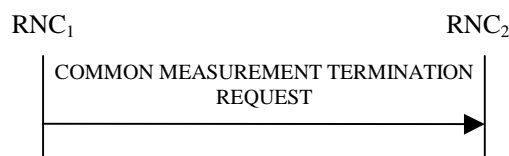
Figure 30D: Common Measurement Termination procedure, Successful Operation
