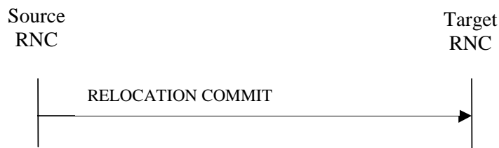
Figure 3: Relocation Commit procedure, Successful Operation
