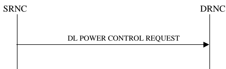
Figure 25: Downlink Power Control procedure, Successful Operation
