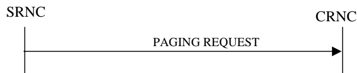
Figure 4: Paging procedure, Successful Operation
