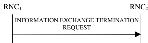
Figure 30I: Information Exchange Termination procedure, Successful Operation
