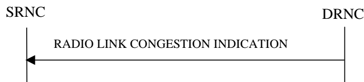
Figure 26C: Radio Link Congestion procedure, Successful Operation
