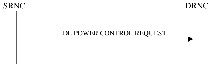
Figure 25: Downlink Power Control procedure, Successful Operation
