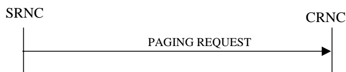
Figure 4: Paging procedure, Successful Operation
