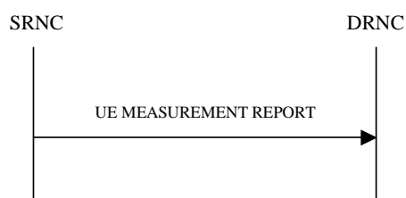
Figure 26H: UE Measurement Reporting procedure, Successful Operation
