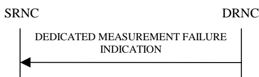
Figure 24: Dedicated Measurement Failure procedure, Successful Operation
