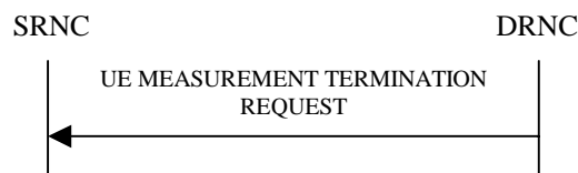
Figure 26I: UE Measurement Termination procedure, Successful Operation
