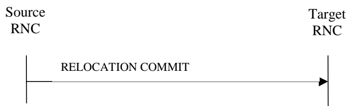
Figure 3: Relocation Commit procedure, Successful Operation
