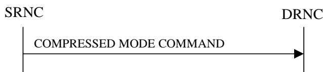
Figure 26: Compressed Mode Command procedure, Successful Operation
