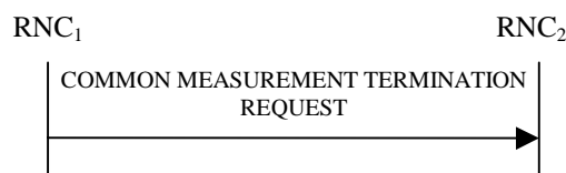
Figure 30D: Common Measurement Termination procedure, Successful Operation
