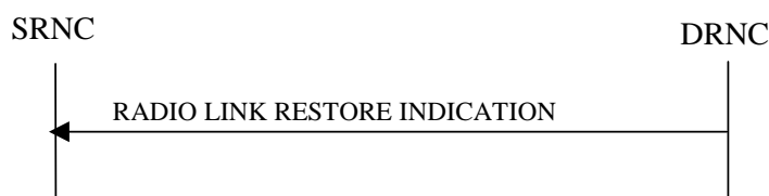
Figure 19: Radio Link Restoration procedure, Successful Operation
