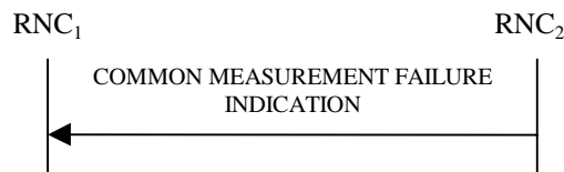
Figure 30E: Common Measurement Failure procedure, Successful Operation
