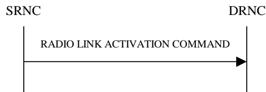
Figure 26D: Radio Link Activation procedure
