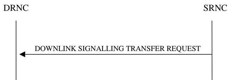
Figure 2: Downlink Signalling Transfer procedure, Successful Operation
